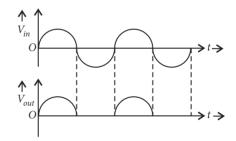
During negative half cycle of input a.c., end A of the secondary winding becomes negative and end B positive. Thus, diode D becomes reverse biased and does not conduct any current. So, no current flows in the circuit. Since electric current through load  $R_I$ flows only during positive half cycle, in one direction only *i.e.*, from A to B, so d.c. is obtained across  $R_L$ .
